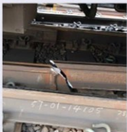
Cracks in railway tracks were found following the Hung Hom derailment in September, causing chaos for passengers.
