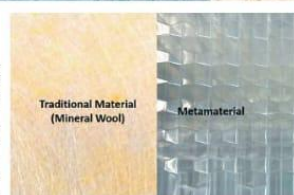
The interlacing air pockets in the layers of plastics work in unison with the plastic layer to form a composite panel with much more effective sound absorption.
